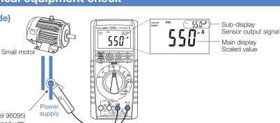
AC/DC clamp-on probe (Model 96095) Reads maximum 60 A when used with the CA450.
