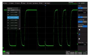
History function can record up to 80,000 frames of waveforms. The recording is executed automatically so that the customer can playback the history waveforms at any time to observe unusual events and quickly locate the area of interest using the cursors or measurements. The failed frames of the Mask Test can be stored as history
