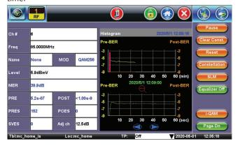
The histogram feature records level, MER, Pre-BER, Post-BER and Error Seconds on a per second or per minute time bucket, for up to 60 minutes. The results are shown in graphical format that allows easy correlation of measured parameters down to one-second resolution.
