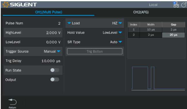
Supports up to 30 pulses, and can set each pulse width and pulse interval.
