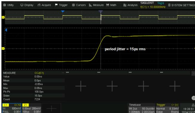
When a Square/Pulse waveform is generated by DDS, there will be a one-clock-jitter if the sampling rate is not an integer-related multiple of the output frequency. EasyPulse technology successfully overcomes this weakness in DDS designs and helps to produce low jitter Square/Pulse waveforms.
