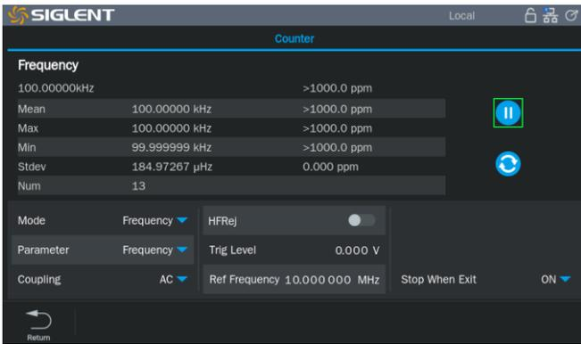
When the counter is in frequency counter mode, it can be used to measure the frequency, period, and duty cycle of a signal. The measurement range is 0.1 Hz ~ 200 MHz.
