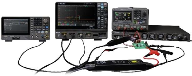
Built-in dual pulse output function, combined with siglent's oscilloscope, can quickly measure the switching parameters and dynamic characteristics of power devices without the need for host computer software.
