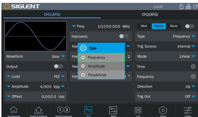
Supports three sweep modes: frequency, amplitude, and frequency and amplitude, making it easy to implement frequency sweep and amplitude sweep tests.
