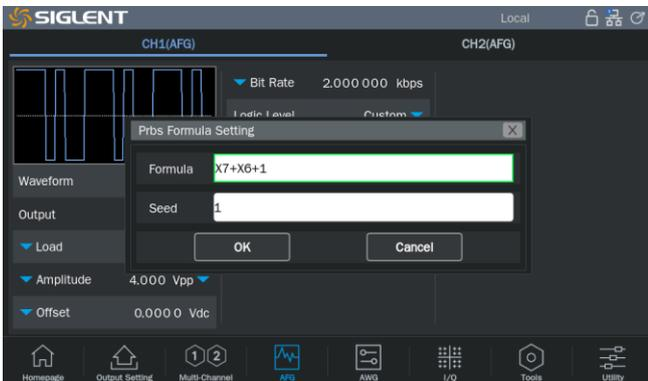
Provides PRBS3 ~ PRBS32 multiple pattern outputs, with a maximum bit rate of up to 120 Mbps. In addition to outputting single-ended signals, the two channels can also be set to differential output.
