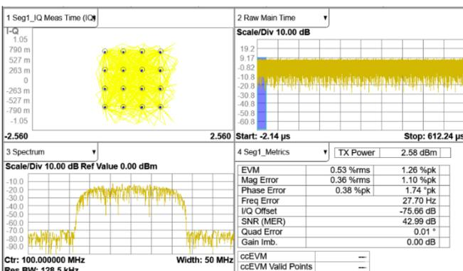
SDG3000X supports baseband or IF signals and can generate IQ signals of commonly used modulation types such as ASK, FSK, PSK, QAM, etc. SDG3000X can achieve excellent EVM performance at any symbol rate in the range of 250 Symb/s ~ 50 MSymb/s. The built-in digital orthogonal modulator can modulate the IQ signal to any frequency in the range of 200 MHz.
