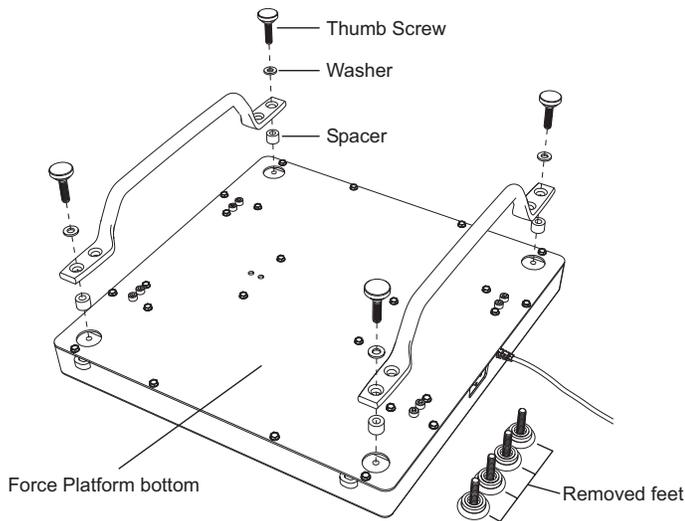
**Handle installation on bottom of Force Platform**
