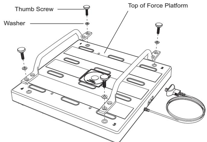
Handle installation on top of Force Platform
