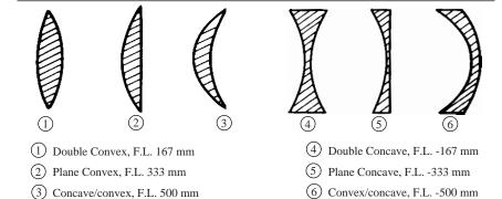
This set of six ground glass lenses provides a useful range of focal lengths for demonstrations and experiments. Each lens is 50 mm in diameter. The diagram above illustrates the geometry of each lens as well as the focal length. The diagrams below illustrate imaging effects of four of the lenses.
